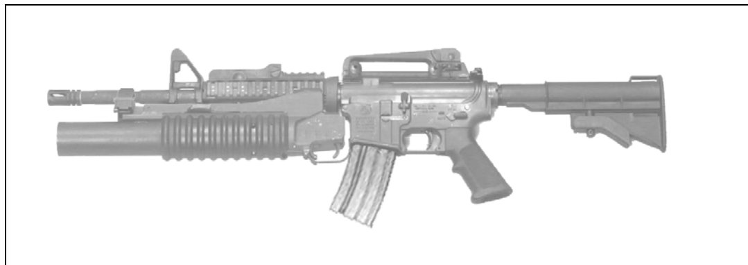
Figure 3-2. M4 carbine with M203A1 (left side view).
